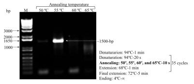
**Figure 4.** Gel electrophoresis was performed for PCR product from the plasmid [MaSp1]8\_pMK-RQ obtained by using different annealing temperatures of 50°, 55°, 60° and 65°C in PCR; details on the right side of the image. The white arrow shows the wrong amplified fragment, bright at 55°C. bp: base pair; M: marker.
