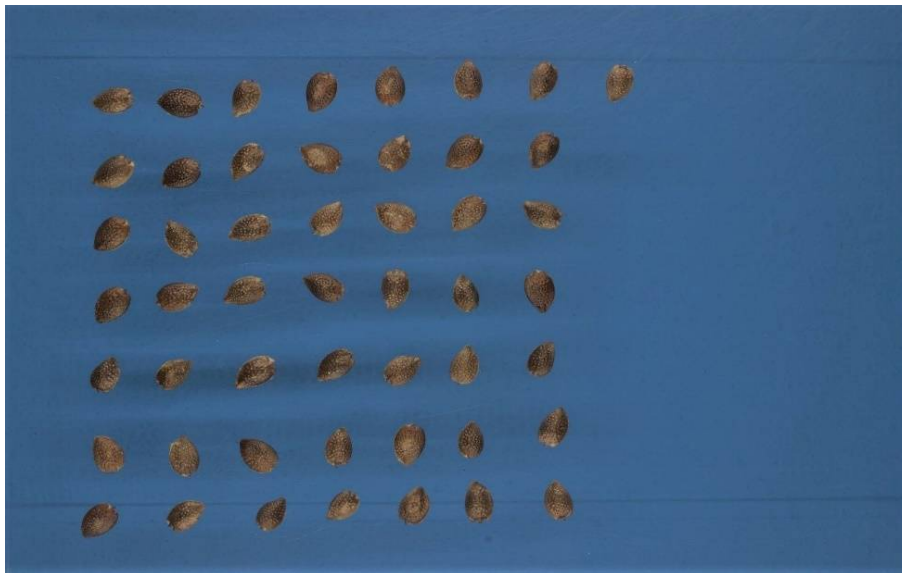
Figure 1. Arrangement of passion fruit seeds on a transparent acrylic tray to collect images using the GroundEye ® seed analysis device.
