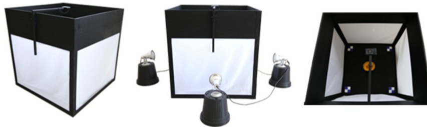
Figure 2. Studio used for the acquisition of images of winter squash fruits for morphoagronomic characterization.
