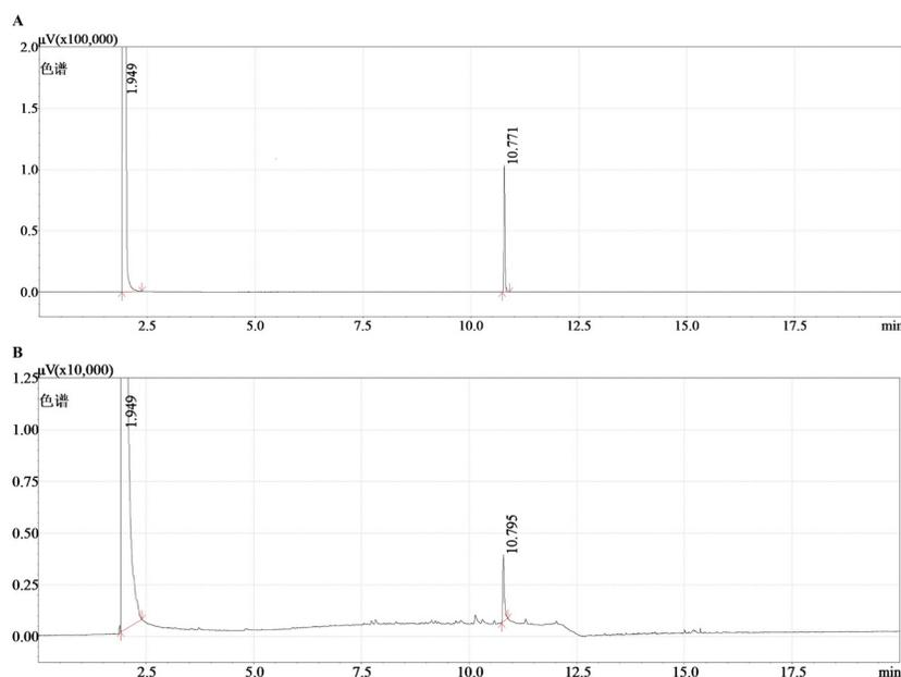
**Figure 1.** Gas chromatogram of the 0.5  $\mu\text{g/mL}$  propamocarb standard. Gas chromatogram of the D9320 sample.
