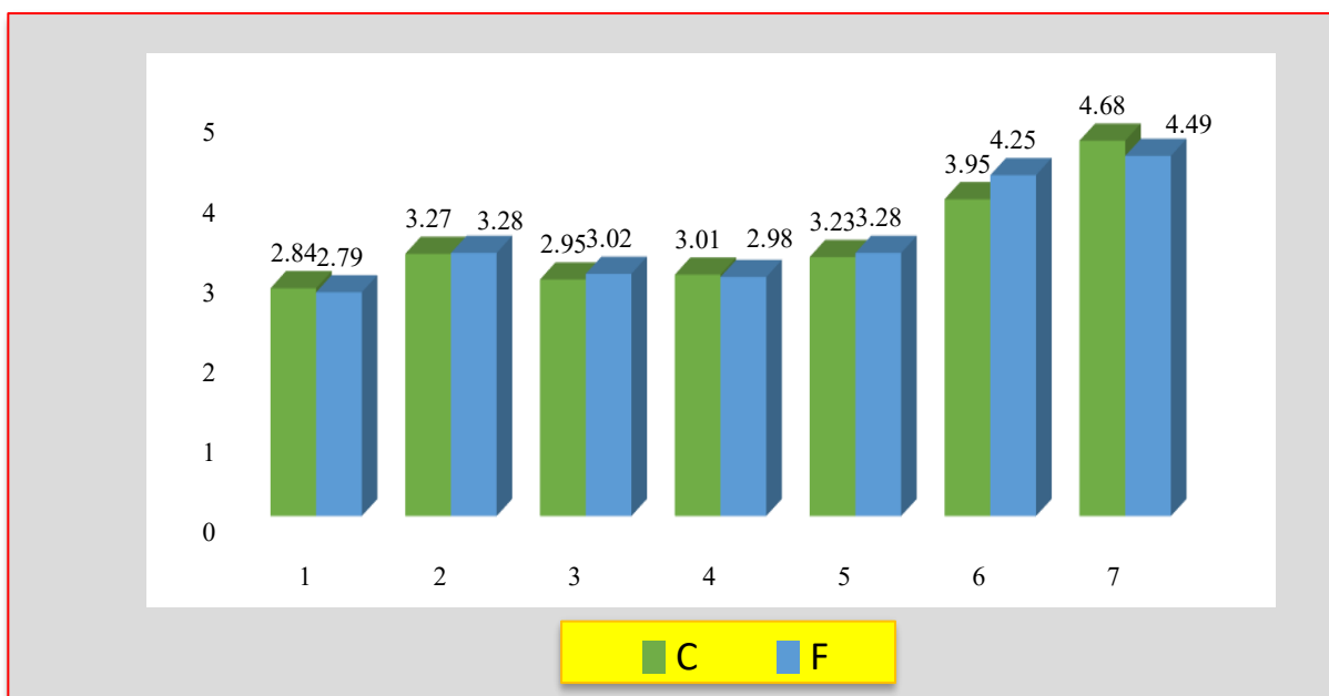
Graph 2: B and E [Pairwise comparison of mean difference of flexural strength between Ivoclar (B) and lucitone (E) groups].
