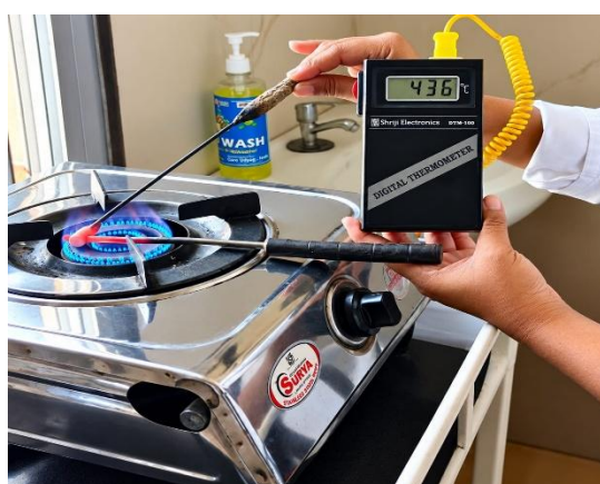
Temperature measured by pyrometer to become red hot
