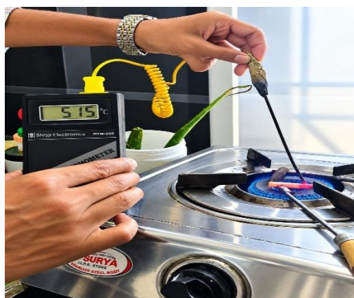
Temperature measured by pyrometer to become red hot
