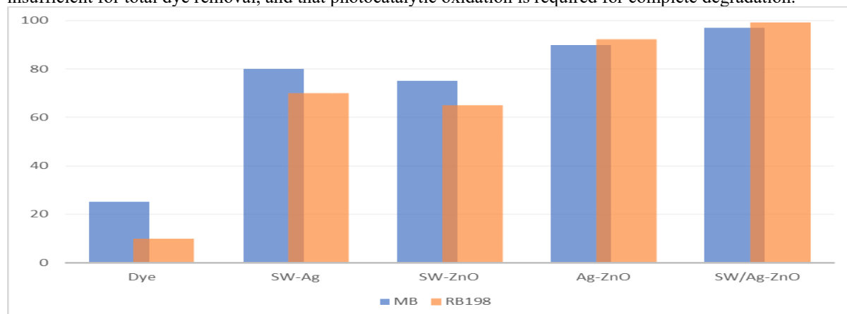
Fig. 10(C). Comparative degradation efficiencies of MB (blue) and RB 198 (orange) across different nanocomposite formulations.
