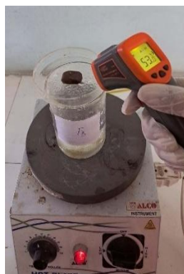
Figure 10: Determination of the softening point of medicated chewing gum using a hot plate and infrared thermometer
