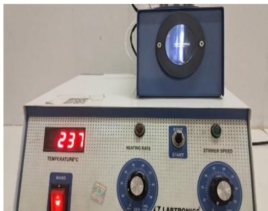
Figure 4: Determination of the melting point of caffeine using a digital melting point apparatus
