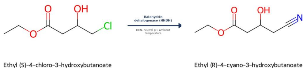
Figure 5. Two-enzyme route to the atorvastatin side-chain intermediate: ketoreductase-mediated asymmetric reduction followed by halohydrin-dehalogenase-catalysed cyanide substitution.
