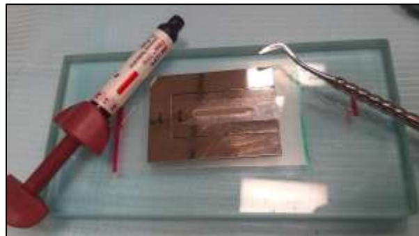
Fig: Flexural Strength specimen - 2mm × 2mm × 25mm length
