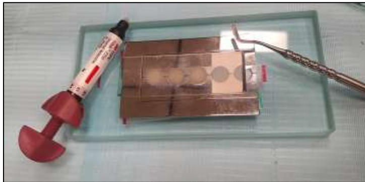
Fig: Compressive Strength specimens - 2mm × 10mm diameter.
