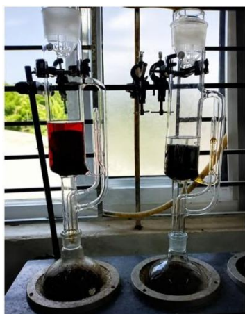
Fig. 5: Soxhlet extraction for GC-MS analysis
