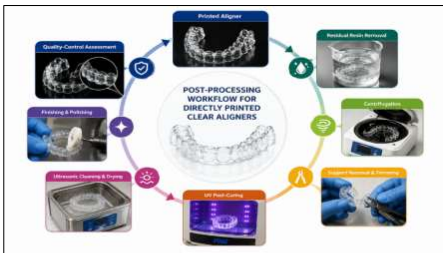
Figure 5. Post-Processing Workflow for Directly Printed Clear Aligners
