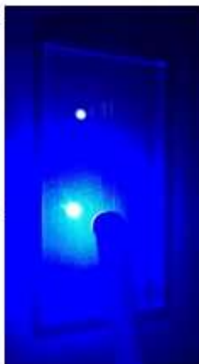
Figure 14. Curing is done with the LED curing light (≥ 1000)
