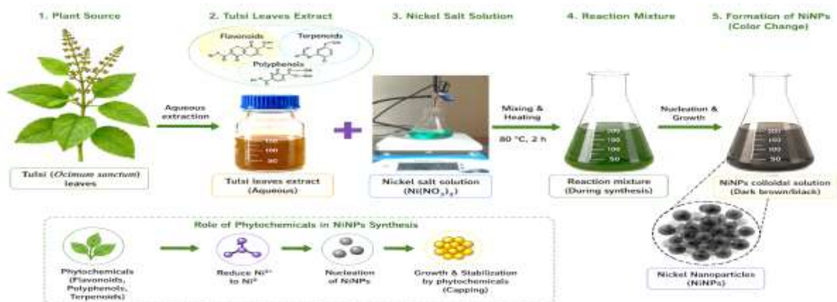
Figure 1. Green Synthesis of Nickel Nanoparticles (NiNPs) Using O. sanctum Leaf Extract
