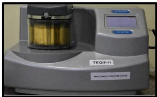
FIGURE 4 : GOLD COATING & SPUTTER COATER MACHINE
