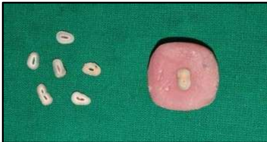
Figure 2- Preparation of dentin discs and Mounting the teeth on acrylic blocks for sectioning
