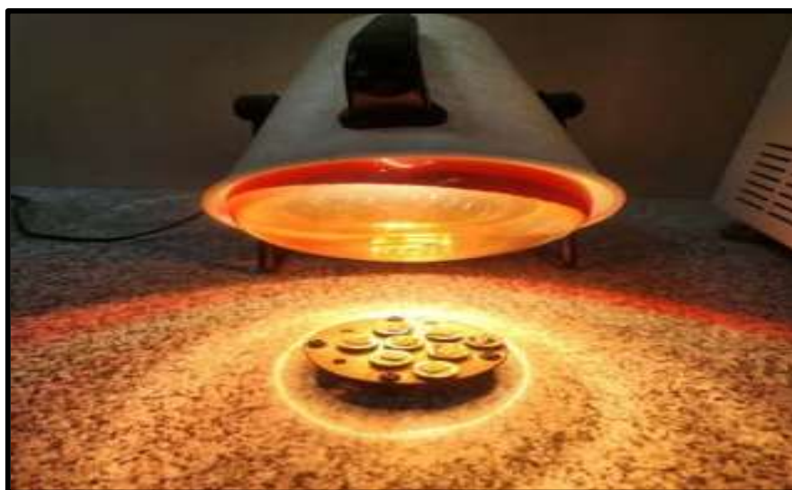
Figure 3- UV radiation for drying of samples
