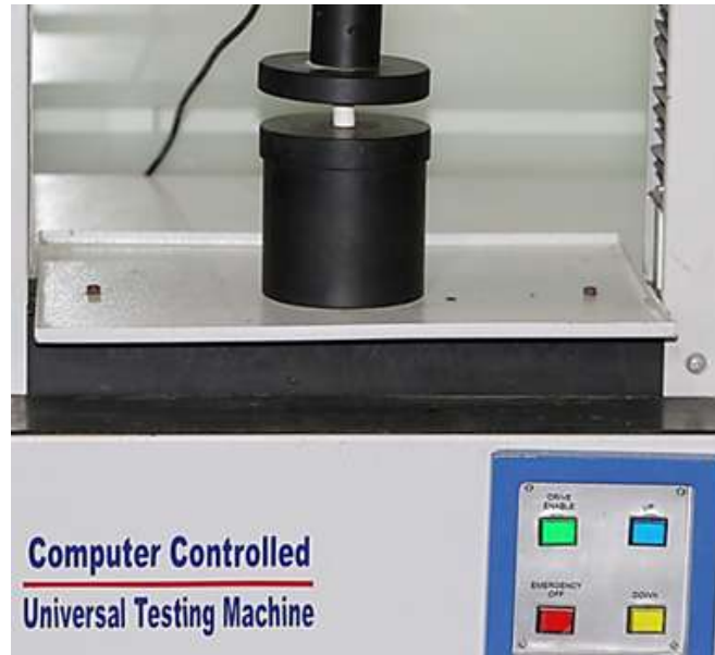
Figure 3: Sample placed in Universal testing machine M 50 – UTM (Hitech Equipment India Pvt)
