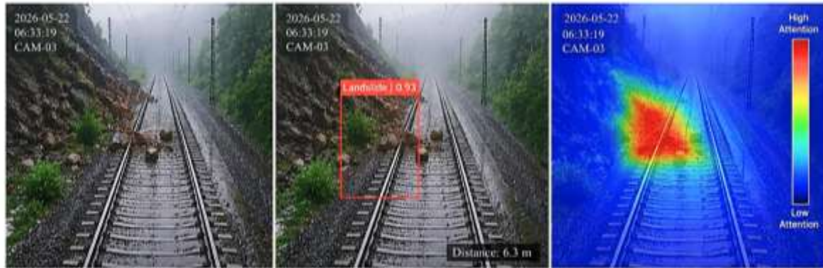
Figure 17. Real-time Landslide (Hazardous Obstacle) Detection on Railway Tracks Using the Suggested YOLO–CNN–LSTM–Attention Model. (a) Original Monitoring Frame, (b) YOLO-Based Landslide Detection and Localization, (c) Attention-Guided Thermal Feature Visualization
