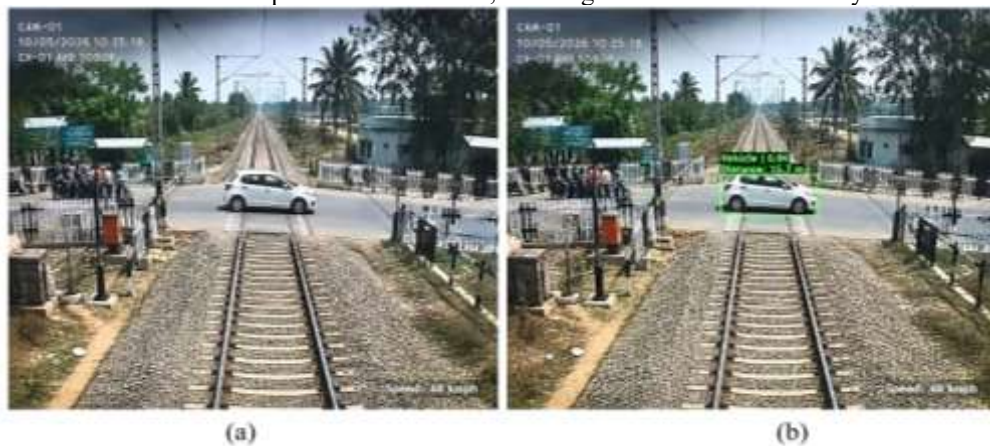
Figure 15: Accurate detection of moving vehicle objects on railway crossings using YOLO under dynamic conditions. a) Original Scene b) YOLO Localization with Enhanced Visualization
