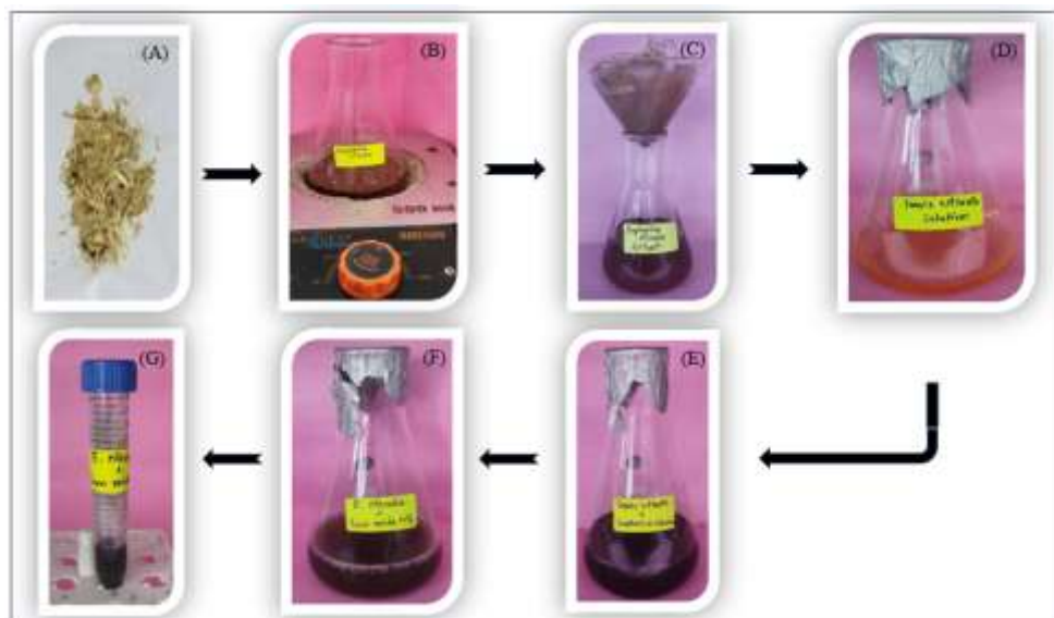
Figure 1: A schematic illustration of the green production of iron oxide nanoparticles using E. nivulia latex extract shows how the plant extract is processed, combined with ferric nitrate solution, filtered, incubated, and a nanoparticle suspension is created.
