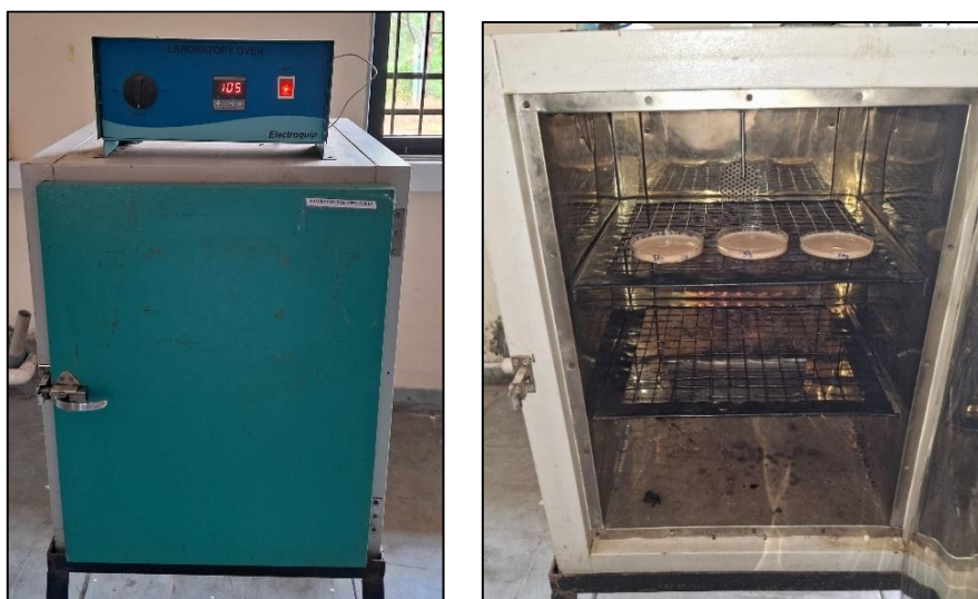
Plate 1 Determination of moisture content in hot air oven
