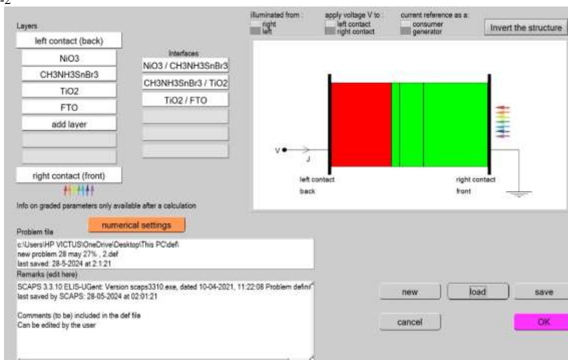
Figure.2: Set-Up Over-View of Layer-Added (SCAPS-1D)
