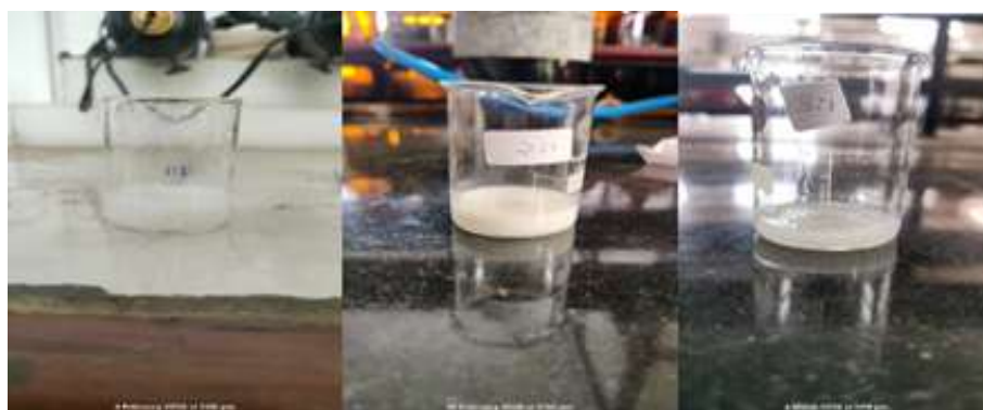
Fig 2. Emulsion formation with oil: surfactant ratio (a)1:1 (b)2:1 (c)3:1
