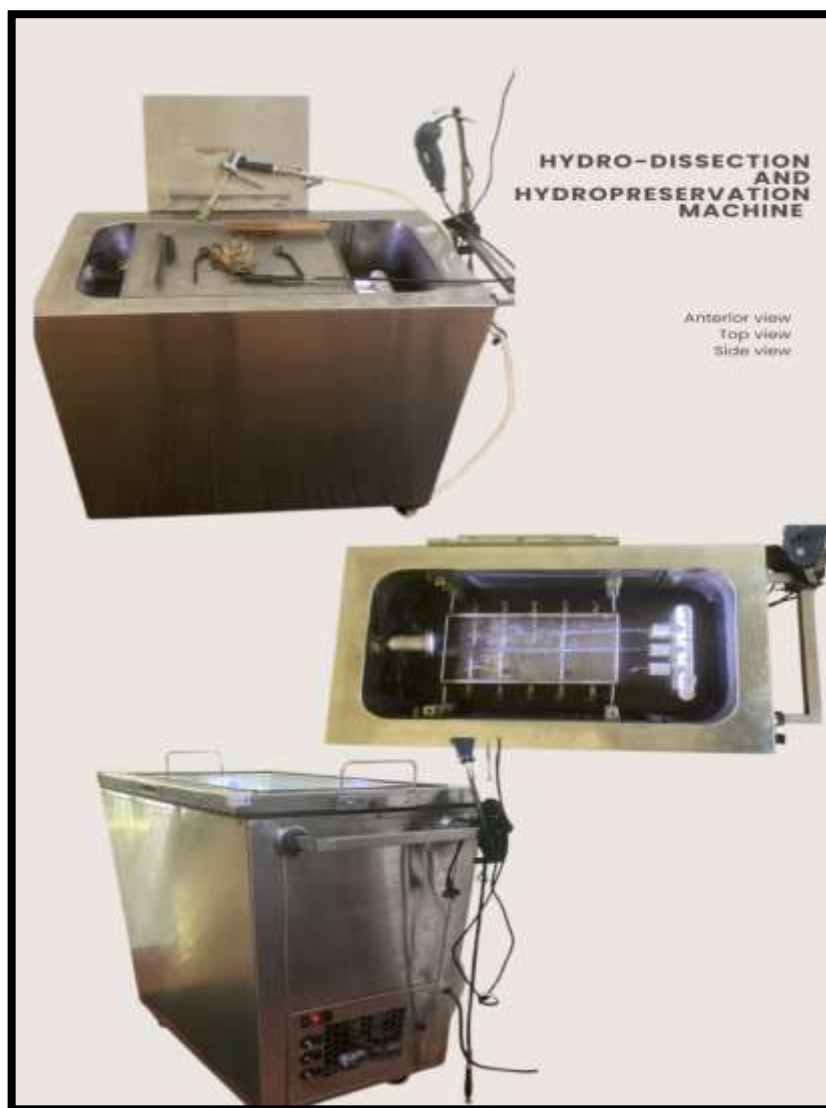
Fig B: The designed hydrodissection and hydropreservation machine in different views, front, top and side view.
