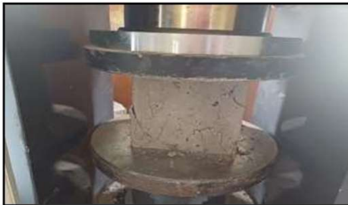
Fig.6 Testing of Compressive Strength using 2000KN compression testing Machine
