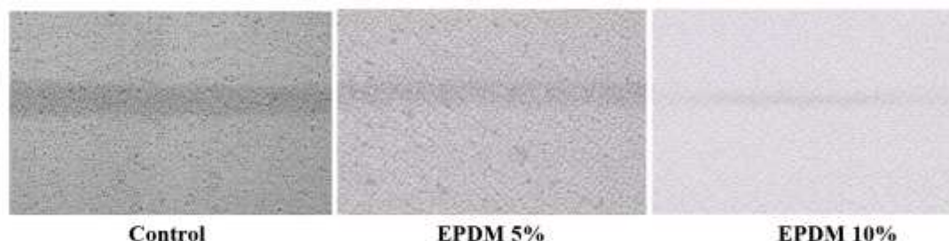
Figure 9: Optical microscopy images showing weld regions of (a) PP/Al 27 + EPDM 5% and (b) PP/Al 27 + EPDM 10%
