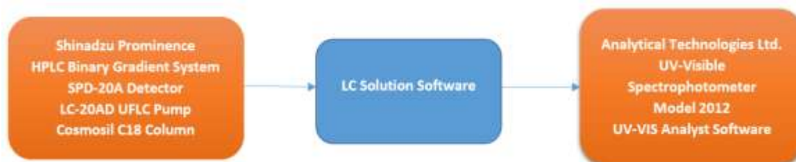
Figure 3. Integrated Analytical System for Quantitative Determination of Pesticides Using HPLC and UV–Visible Spectrophotometry (ChatGPT).
