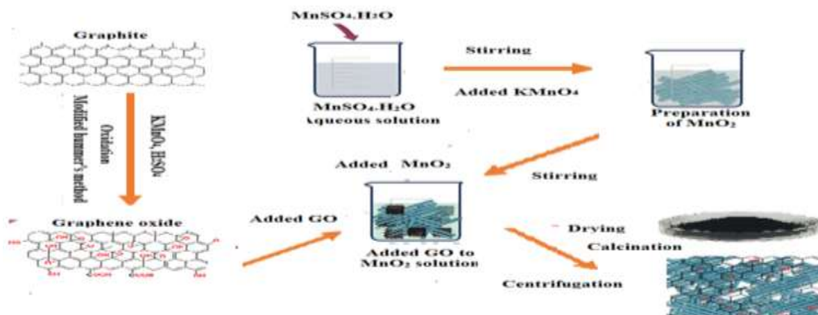
Figure 1. (a) Synthesis of graphene oxide (b) Schematic diagram of preparation of GO– \text{MnO}_2 nanorods
