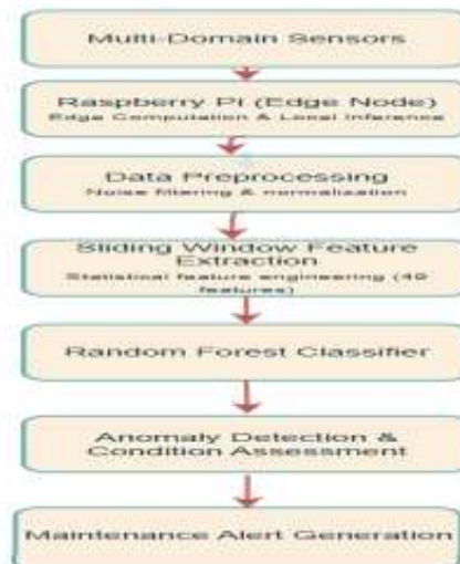
Figure 1 . Layered architecture of the proposed edge-intelligent condition assessment framework.
