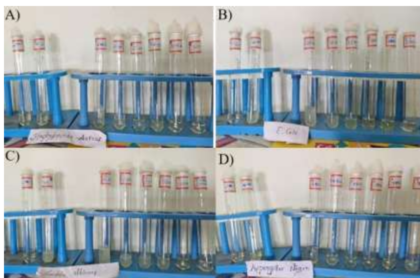
Figure 6. Determination of minimum inhibitory concentration (MIC) of optimized Allium sativum oil hair gel formulation (F3) against (a) Staphylococcus aureus , (b) Escherichia coli , (c) Candida albicans , and (d) Aspergillus niger .
