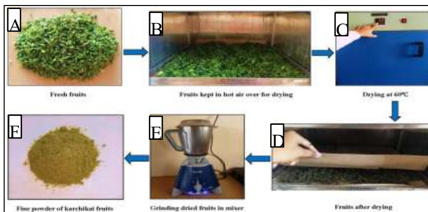
Figure 1. Flow chart of drying and powdering of Karchikai fruits 1A. Fresh fruits collected and cleaned, 1B. Fruits kept in hot air oven for drying, 1C. Set the drier at 60°C, 1D. Oven dried fruits, 1E. Grinding the dried fruits in grinder, 1F. Fine powder of karchikai fruits
